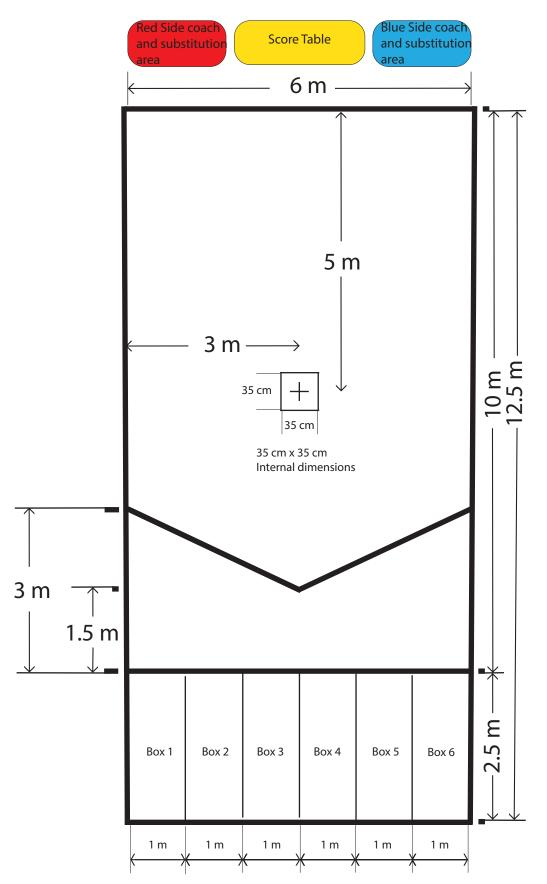
Tape Guidlines--Use wide (approx 2in) tape for the exterior lines, throwing line and V line. Use narrow (approx 1in) for the throwing box dividers, the cross and the target box.
